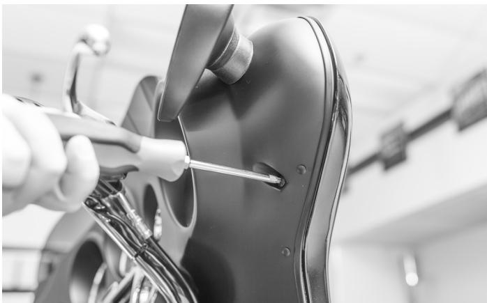
Once you have the windshield set aside, remove the remaining screws on the inside of the fairing. This will allow you to remove the front fairing.
