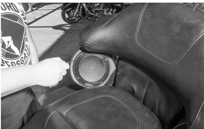
Place the grille over the speaker and attach with the included screws to mount to the pod.
