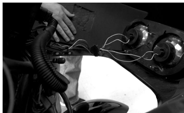
Pull the fairing toward the front of the bike and up to release it from the fairing mounts. Unplug headlight harness and set fairing aside.
