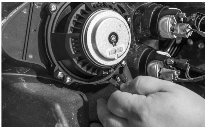
Connect the speakers by sliding the speaker wire connector over the speaker terminals
