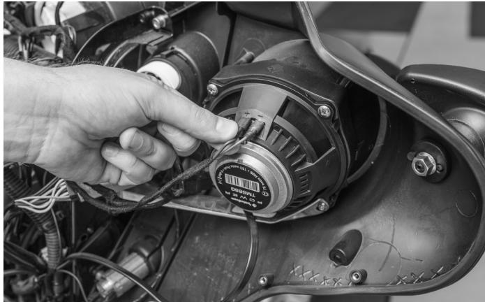
Connect the speakers by sliding the speaker wire connectors over the speaker terminals
