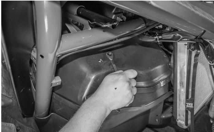
Install using the supplied bolt through the top of the enclosure. The bolt will go through the drilled 5/16" hole. Secure with the supplied nut.
