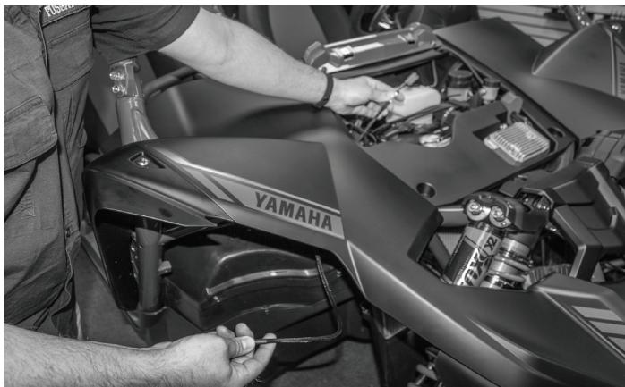
Take the speaker wire harness and run from the RFYXZ-K8 or RFYXZ-PMXDK harness under the hood to the holes drilled in the foot well.
