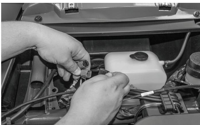
Once both speaker pods are installed and the harnesses are ran, locate the front speaker output connections in the RFYXZ-DK radio harness or the RFYXZ-K8 harness and remove the watertight plugs.
