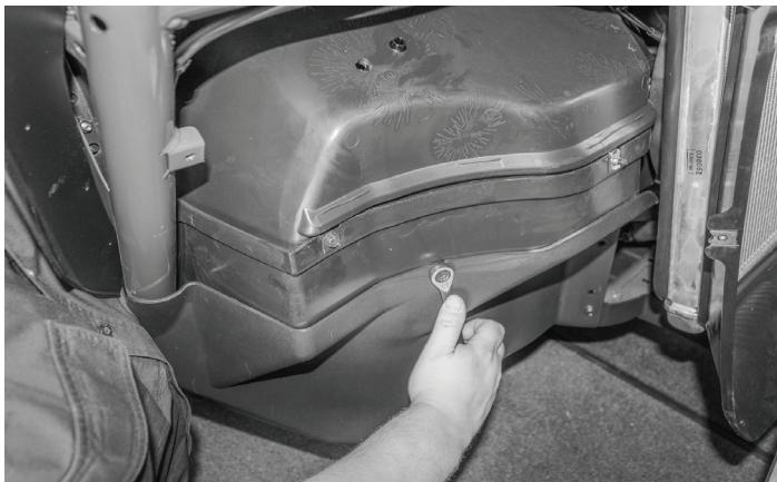
Finish securing the speaker pod in place with the (2) bolts used earlier.
