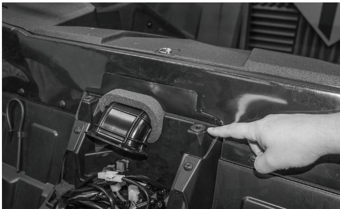
NOTE: When removing, be sure to make sure the rubber grommets are in good condition and inserted correctly. If they are not installed properly, the center console will not engage the correct way or attach securely.
