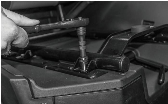
There are (4) mounting bolts holding the seat frame in place. Remove these bolts using a 12mm socket and ratchet. Then, lift the seat assembly out.
