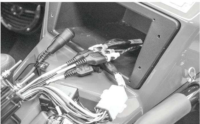
Plug the RCA's from the main harness into the back of the PMX-2 and slide radio into the center console. Secure dash kit to the center pocket once everything is connected.
