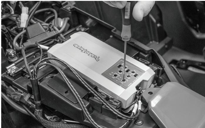
Once the system checks out, set the gains using the Clip Indicator lights on the amplifier.
