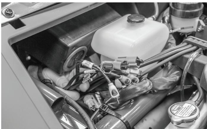
Pass the wire harness through the transmission tunnel leaving the harness under hood.
