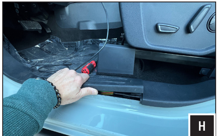
H. Run the subwoofer audio wiring (not included) from the subwoofer to the amplifier location.
