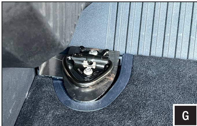
G. Line up the lower housing bracket and factory tie down anchor above the spacer. Use (2) M8x1.25x40 button head bolts and washers to firmly secure the Bronco subwoofer enclosure.
