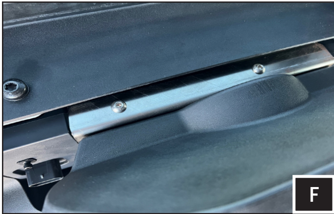
F. Mount the Bronco sub enclosure upright and line up the upper bracket screw holes to the body bracket pem nuts. Use (2) M8x1.25x20 button head screws and washers included in kit
