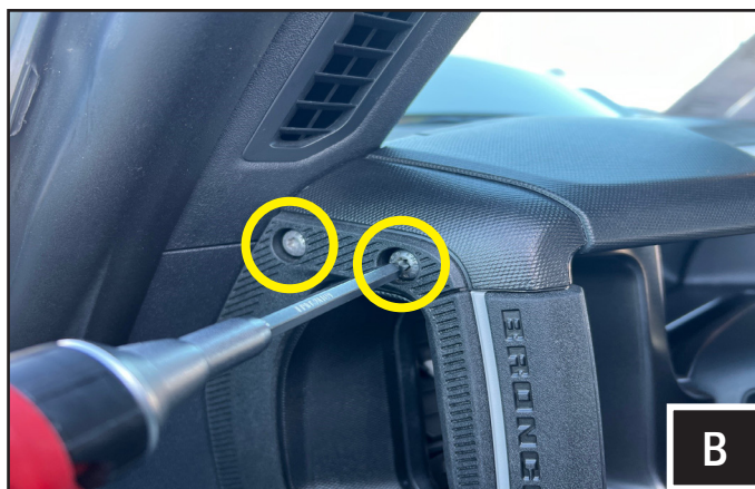
B. Remove the (2) factory screws on the driver side grab handle trim and set aside.
