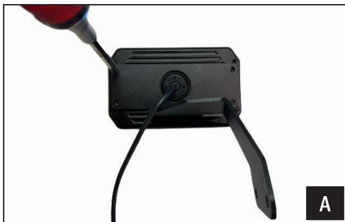
A. Mount the ALPHA12 Controller to the bracket (B-MB3274) using (4) thread cutting screws (B-S3262).
