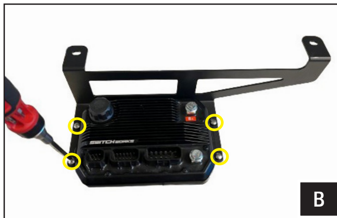
B. Mount the ALPHA12 brain module to the brain bracket (B-MB3277) using (4) M5x10mm pan head screws (B-S1158).
