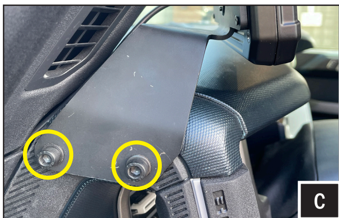
C. Secure the B-MB3274 bracket to the factory grab handle trim using (2) M6x35mm socket head cap screw and M6 flat washers included in the kit. Tuck the cable along the trim seam and run to the engine bay.
