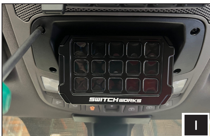
I. Mount the ALPHA12 overhead fascia with the controller to the overhead bracket using the #7-19x.75" screws [x4] (B-S1656).
