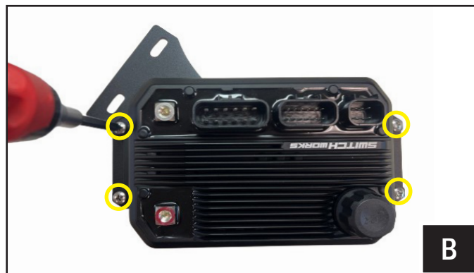
B. Mount the SWITCH Works brain module to the B-MB3192 bracket using the supplied M5x10mm screw (x4).
