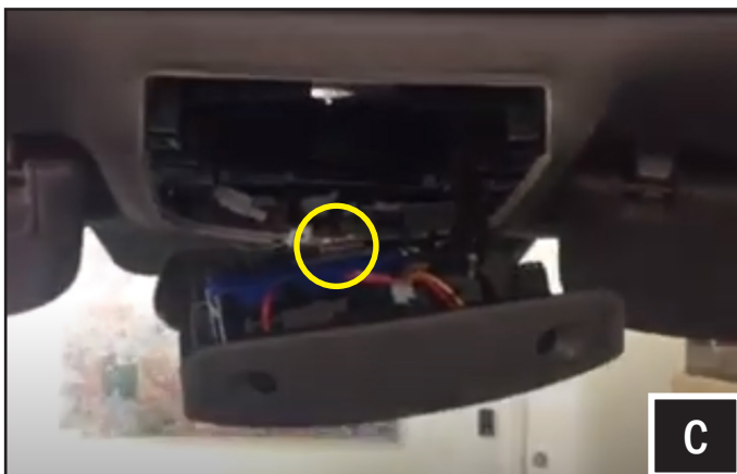
C. Unplug the connector(s) to complete the removal of the console.
