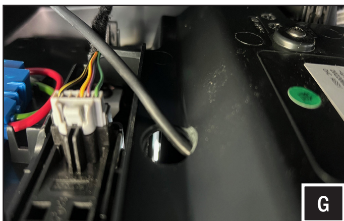
G. the provided 4-40x.375 thread cutting screws (B-S3262). Route the controller cable through the hole and run it along the headliner towards the A pillar.
