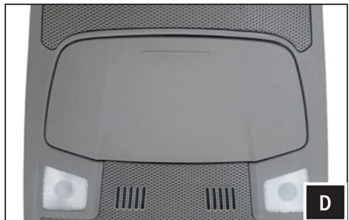
D. Carefully remove the sunglass holder.
