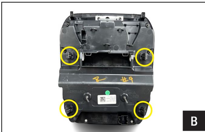
B. Note that there are 4 clips that secure the overhead console to the headliner.
