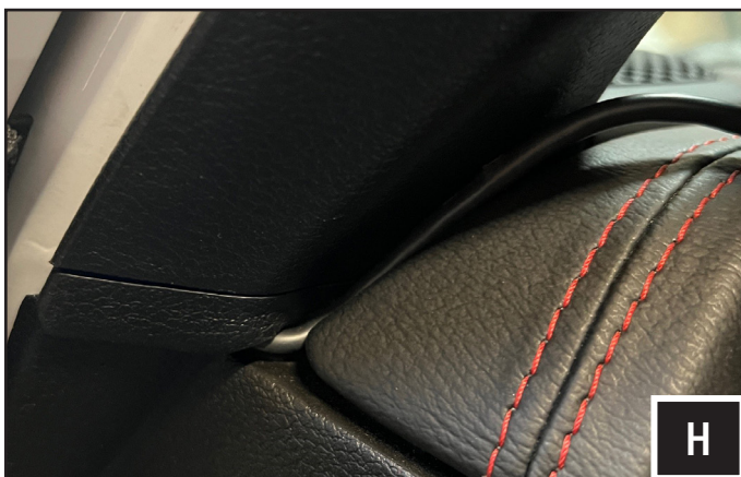
H. Run the cable through the A pillar and to the engine bay.
