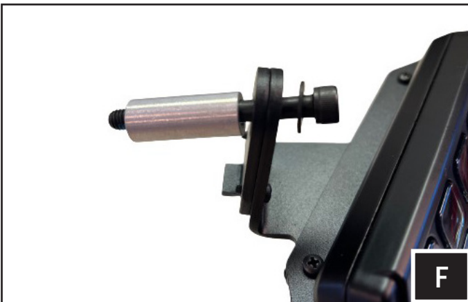
F. Prepare to mount the ALPHA12 controller to the grab handle using the supplied M6x55mm screw, flat washer and aluminum spacer.
