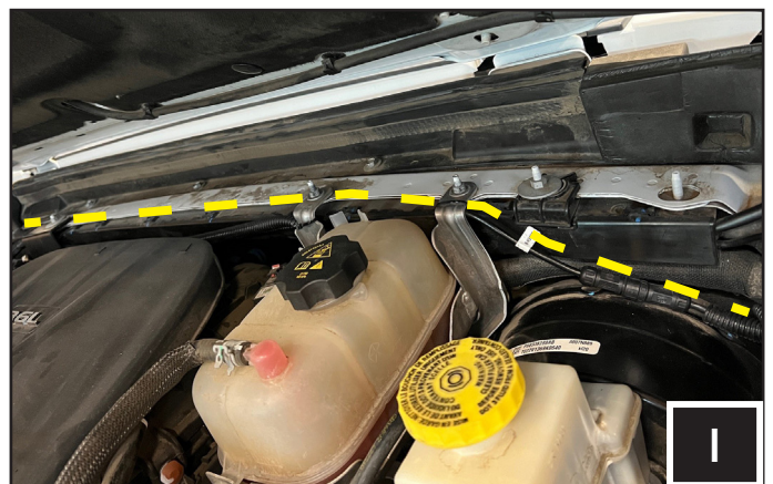
I. Use the supplied 3 ft. controller extension cable and run it along the firewall towards the passenger side of the engine bay. Use zip ties to hold it in place.
