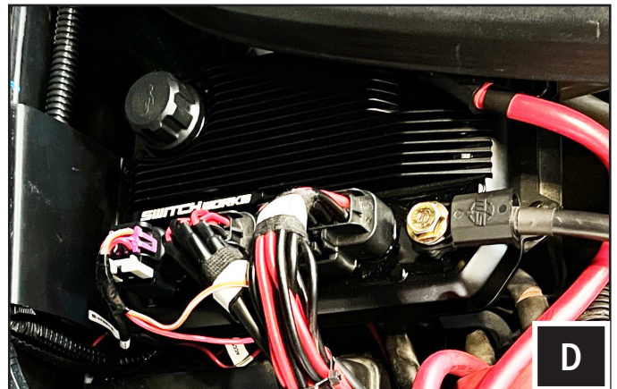
D. Connect the accessories to be used to the High and Low current harnesses and plug the harnesses to the brain module. NOTE that the 15 button controller MUST be plugged in to the module before connecting the power and ground cables to the battery. Snap on the terminal cover to the module's + terminal.
