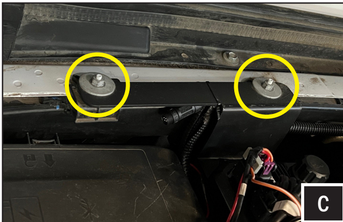
C. Use the factory bolts and washers on the firewall to mount the bracket.
