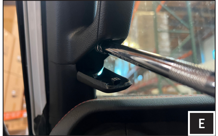
E. Remove the factory grab handle screw using a 10mm socket wrench.
