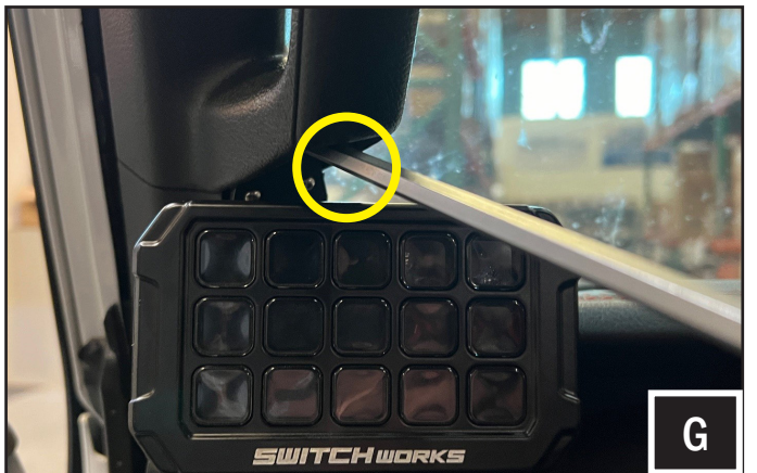
G. Mount the ALPHA12 controller bracket to the factory grab handle using a 5mm Allen wrench. Refer to picture on F.
