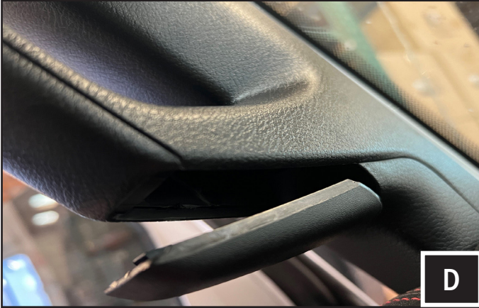
D. Remove the bottom screw cover cap on the driver side grab handle.
