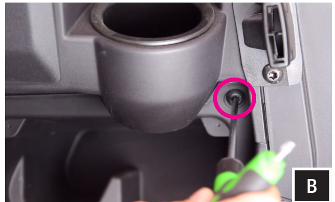
B. Remove factory T40 torx screws located from the front of the dash next to the cup holders.
