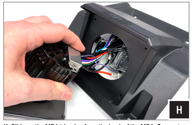
H. Slide on the MR1 trim ring from the back of the MR1. Connect the MR1 and all related accessories. Place the MR1 into the dash mount. When placing the MR1 into the dash mount, feed slack wiring back into the dash cavity cut out. This will allow for proper fitment of the MR1.
