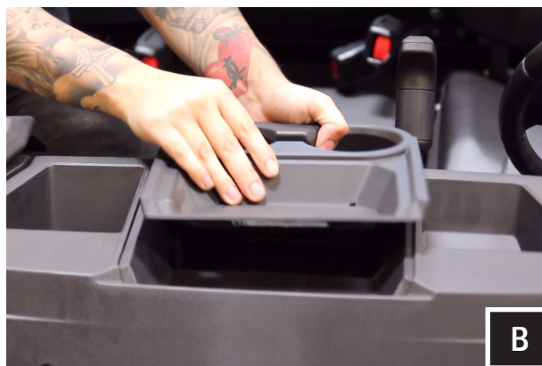
B. With push pins extracted, lift to remove the cup holder.
