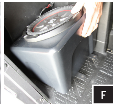
F. With the bracket secured to the floorboard, place the enclosure in front of the floorboard bracket. To allow proper engagement, tilt the enclosure back slightly and slide its bottom bracket into the floorboard bracket catch.
