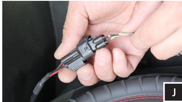
J. Connect sub to harness B-H2702.
