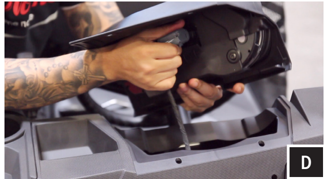
D. Lift and disconnect gauge cluster for removal.
