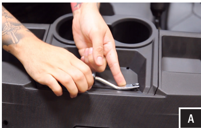
A. Use a panel tool to extract push pins on the top of the center cup holders.
