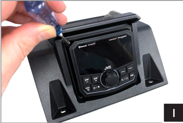
I. Secure the MR1 with the (4) M3.5 screws provided with the MR1.
