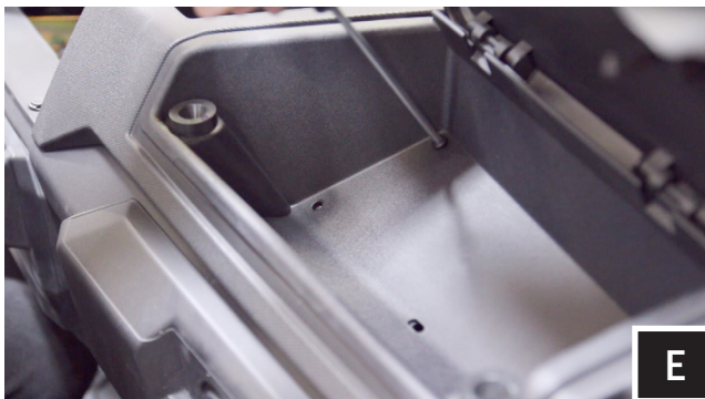
E. Unscrew (4) torx screws located in upper glove box and remove box.
