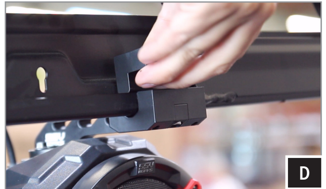
D. Slide the top mount for the clamp into the top crossbar notch and line up screw holes.
