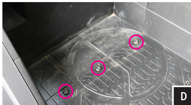
D. Located on the floorboard to the right of the battery compartment, remove the (3) T40 torx screws circled in pink.
