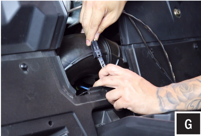
G. Take the B-H2936 rear speaker harness and plug into the B-H1913 & B-H1912 rear audio extension and RGB extension harnesses.
