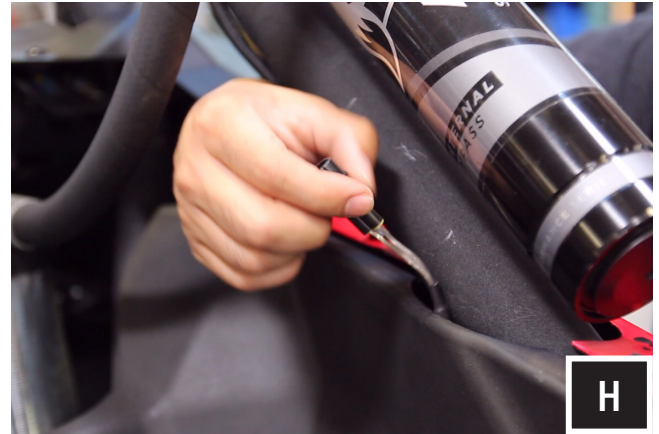
H. Route the rear speaker and RGB extension harnesses (B-H1913, B-H1912, B-H2934 & B-H2933) along the factory wires towards the amplifier and LIT-CC location.
