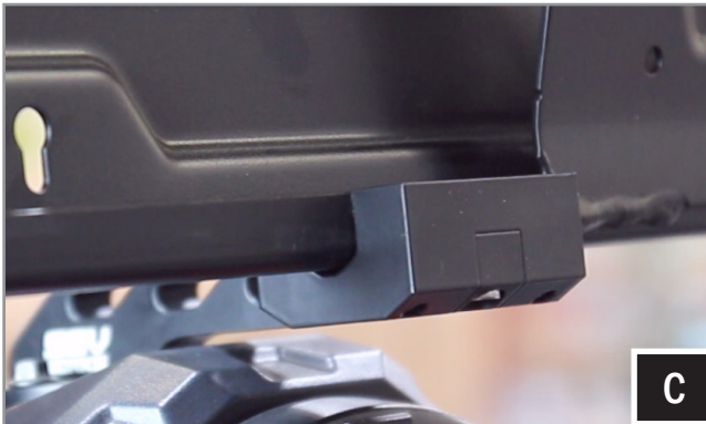
C. Position the clamp underneath the rear crossbar
