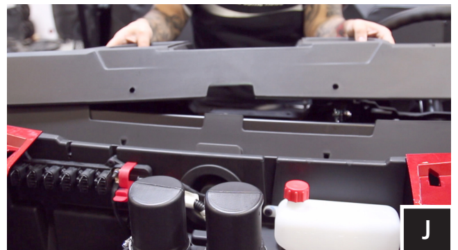
J. Lift to remove the dash.
