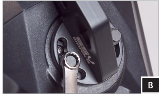
B. Loosely install the clamp base to the cage mount pod with the two (2) M6 Hex head bolts and washers, place the cage mount pod in the desired mounting location and tighten the hex head bolts using a 8mm wrench.
