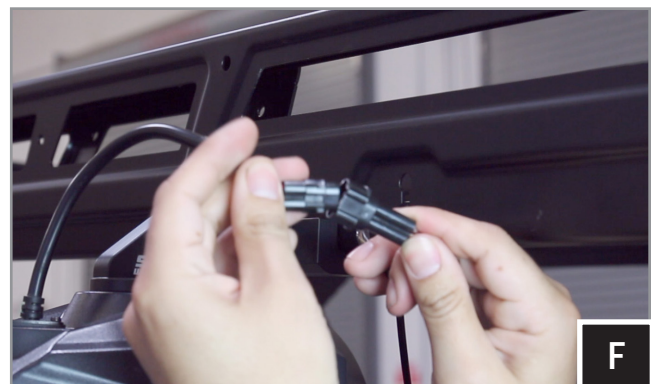
F. Plug the rear cage pod pigtail to the B-H2936 rear speaker harness.
