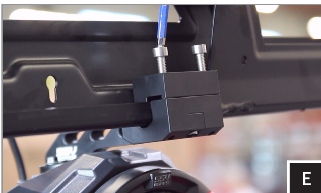
E. Place screws in the clamp and use a 5mm hex driver to tighten the bracket
