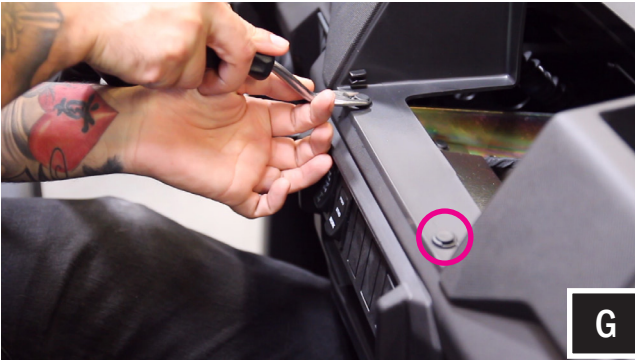
G. Extract push pins exposed from cup holder removal.
