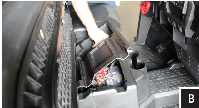
B. Flip up passenger seat and remove center tray to access battery. Disconnect the negative battery cable from the battery.
