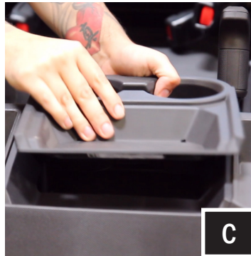
C. With push pins extracted, lift to remove the cup holder.
