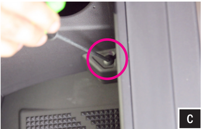
C. Remove factory T25 torx screws located underneath the dash.
