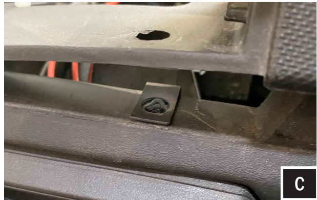
C. Using a panel removal tool gently lift the existing plastic panel on the center dash support. Install the two (2) supplied U-Nut clips by sliding them onto the bottom of the center dash panel support and align holes as needed.
