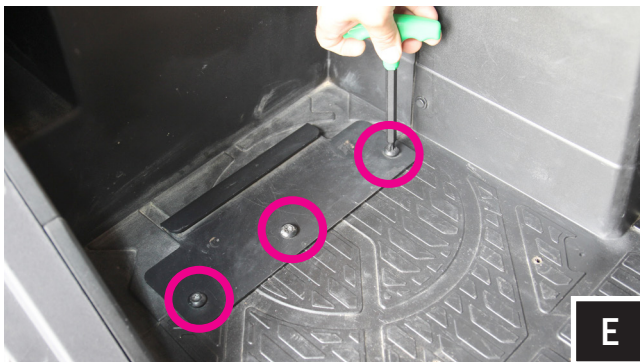
E. Place SSV bracket B over the factory screw holes and refasten down with the (3) factory T40 torx screws removed in the previous step.
