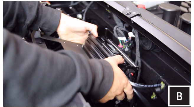
B. Move the factory wiring to the rear of the dash cavity. Place the RG4 Amp mounting plate in the former location of the factory bracket.
