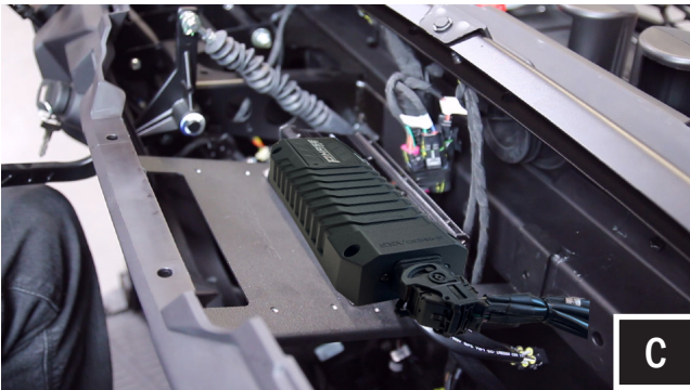
C. With the RG4 Amp mounting plate set in place, check for any pinched wiring.
