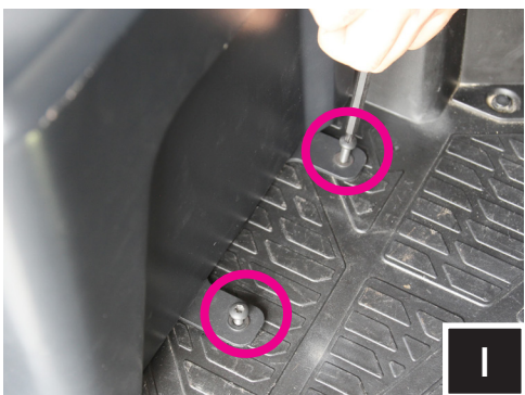
I. Re-install the sub-enclosure. Secure the front mounting tabs with the kit provide T30 torx self-tapping screws.
