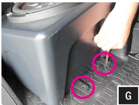
G. With the brackets seated into one another, use the front mounting tabs as a template to mark with a scribe or punch the needed placement to drill pilot holes.
