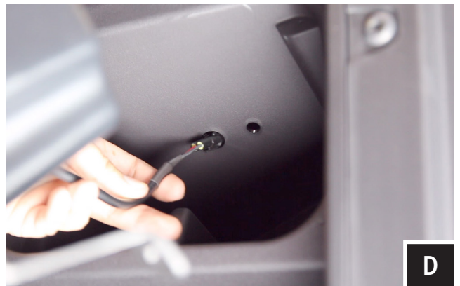
D. Located on the inside top of the pocket you will have two holes, route speaker wire through the larger hole. The smaller hole will be used to mount the pod in Step P.
