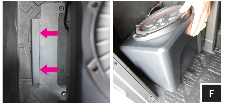
F. With the bracket secured to the floorboard, place the enclosure in front of the floorboard bracket. To allow proper engagement, tilt the enclosure back slightly and slide its bottom bracket into the floorboard bracket catch.
