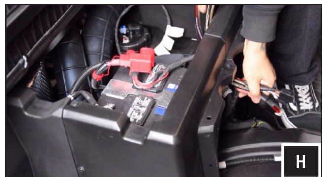
H. Follow the air ducts and factory wiring and feed cables towards the battery compartment. Use the provided zip ties to secure the cables to the factory wiring, away from the drive shaft.
