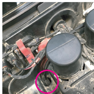
F. With the cables now through the firewall, route them down and into the vehicle cabin. NOTE: A 1" hole will need to be drilled to run the cables down the front of the chassis.
