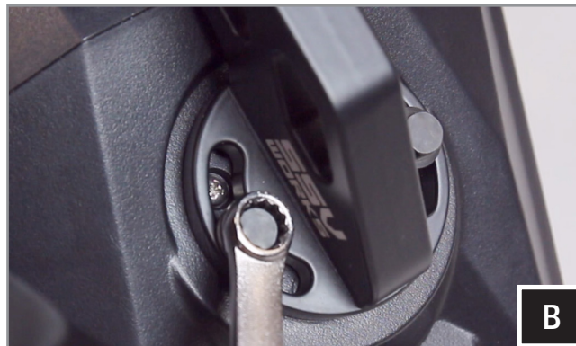
B. Loosely install the clamp base to the cage mount pod with the two (2) M6 Hex head bolts and washers, place the cage mount pod in the desired mounting location and tighten the hex head bolts using a 8mm wrench.
