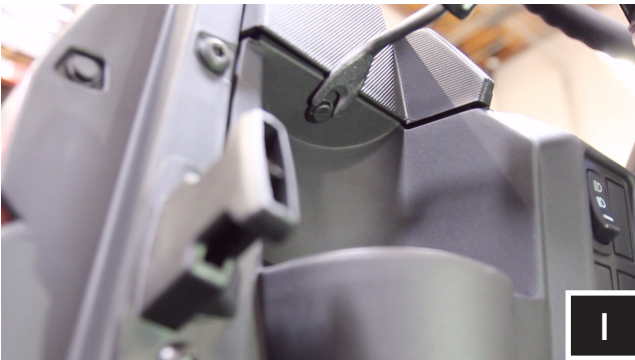
I. Extract push pins located above driver and passenger side cup holders.
