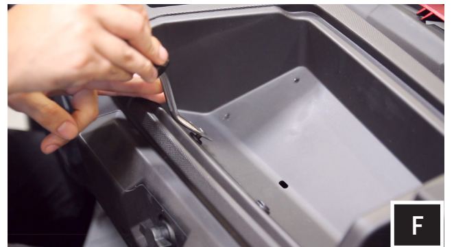
F. Extract push pins that are now exposed from removing the upper glove box.
