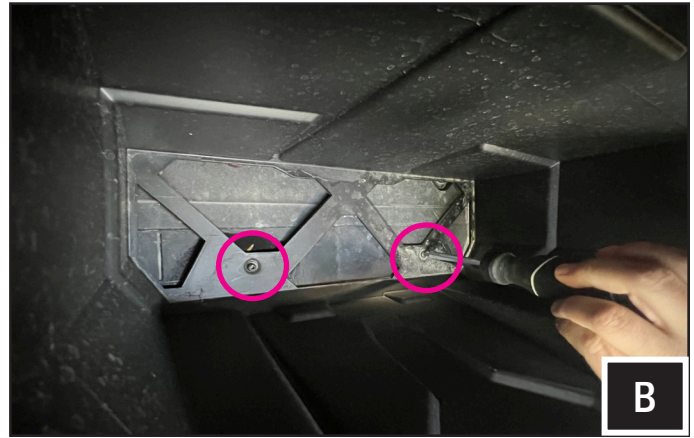
B. Remove the driver side underseat storage bin by removing the 2 screws fastened to the floor.
