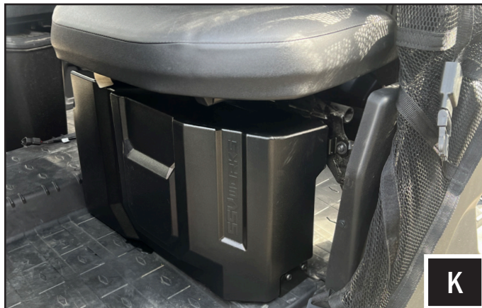
K. Once all the screws are lined up, tighten all 4 screws to secure the Defender sub enclosure to the vehicle.
