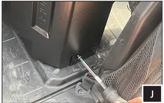
J. Use (2) of the supplied screws [B-HPM616-4] to fasten bracket A to the Defender sub enclosure. Do not completely tighten yet.
