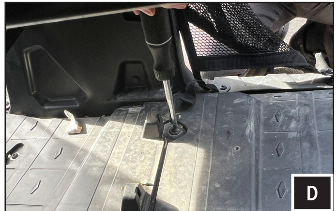
D. Remove the T-30 Torx floor screw.
