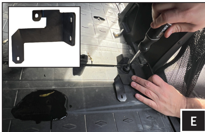
E. Mount bracket A on the floor using the factory screw removed on step D.
