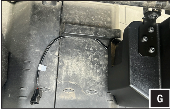
G. Place the Defender sub enclosure under the seat and run the cable towards the amplifier location.
