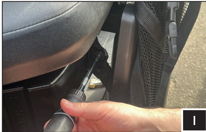
I. Use the factory screw to fasten bracket B to the other U-Nut on the right side of the vehicle. Do not completely tighten yet.
