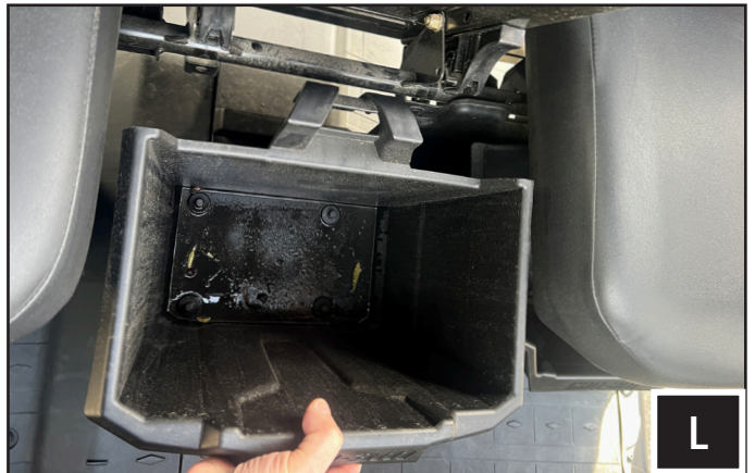
L. Hook back the middle seat storage bin. This completes the installation of the Defender Subwoofer Enclosure.
