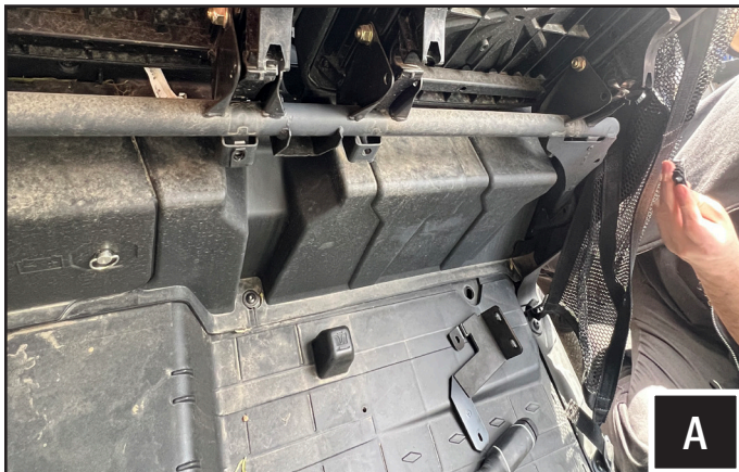
A. Lift driver seat. Note that the vehicle in this installation did not have an underseat storage bin.
