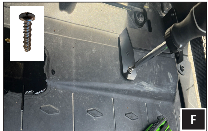
F. Fasten the front end of bracket A using the thread forming screw (B-S3367) included in the kit.
