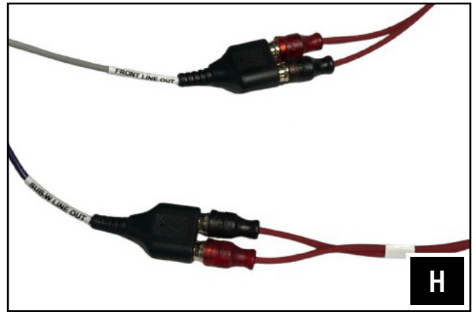
H. Connect the B-HRCA3 RCA cables to the JVC radio's Front and Sub W Line Outs.
