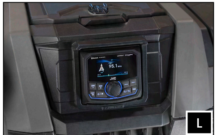
L. Fasten the (4) dash screws center the trim ring on the MR1 and firmly press down until each side and corners click into place. Replace all factory panels.
