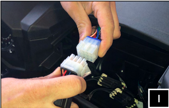
I. Connect the MR1 power harness to the radio harness. Use the provided universal antenna (B-H1249) if the vehicle does not have an antenna.
