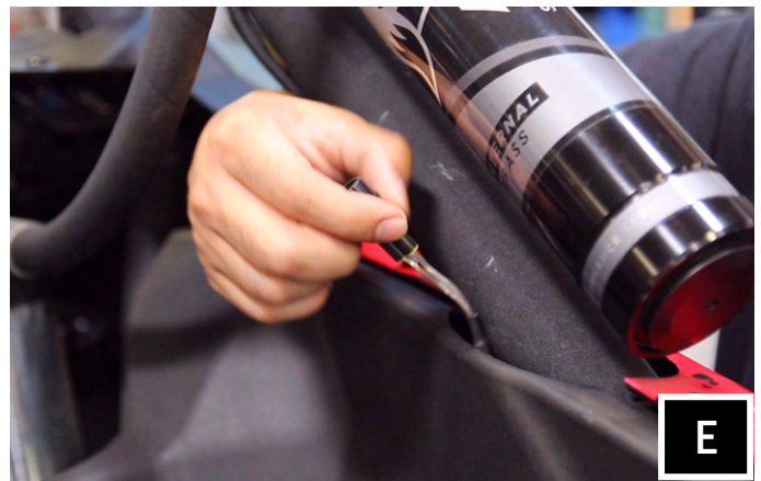
E. Route the rear speaker harness (B-H1909) along the factory wires in the engine compartment and pull up through the small space between the bed panel and cage tubing on both passenger and driver sides.
