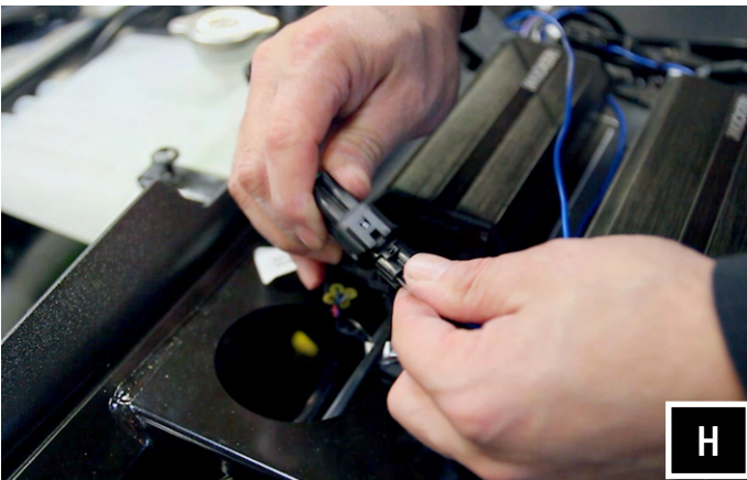
H. Connect the subwoofer cable to the 500.1 amplifier output.
