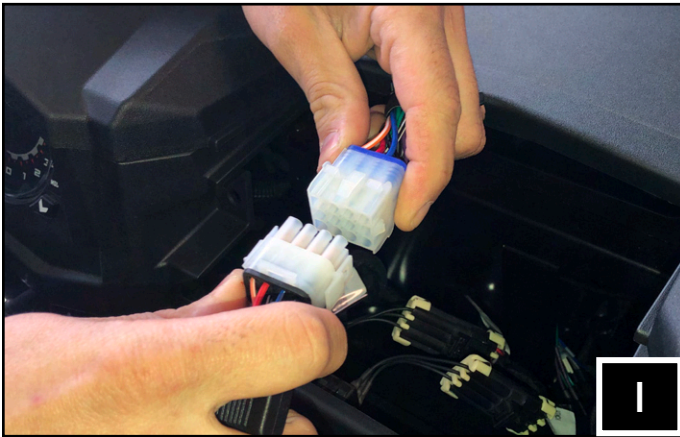
I. Connect the MR1 power harness to the radio harness.
