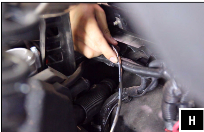
H. Route the rear speaker harness (B-H2195) and RGB harness (B-H2936) along the factory wires in the engine compartment and pull up through the small space between the bed panel and cage tubing on both passenger and driver sides. Plug in the connectors to the cage pods. Run the other end of the audio extension harness to the amplifier location and the RGB extension harness to the LIT-CC location.
