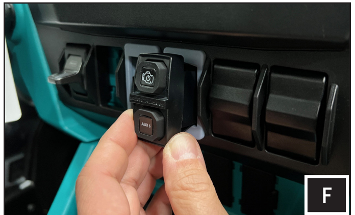
F. Route the cable and Insert the RS6 Switcher Controllers into empty rocker switch openings on the dashboard.
