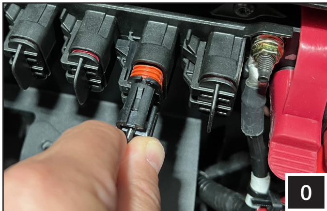
O. For vehicles with the Pulse busbar, plug in the Pulse Connector Pigtail (B-H1752), crimped on step H, to the busbar.
