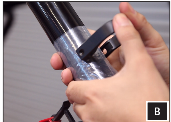
B. Slide in the clamp on the cage tube and remove the plastic.
