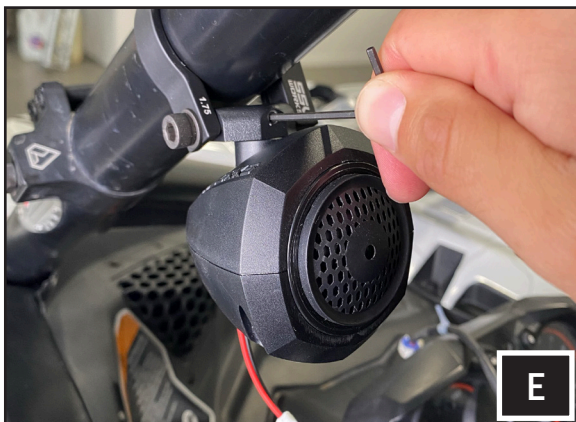
E. Adjust the tweeter pod to the desired angle and fully tighten the set screw and M6 allen socket head bolt.
