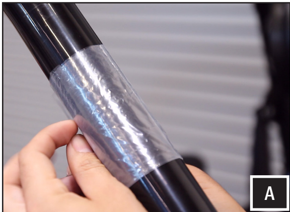
A. Select the correct cage clamp size. Wrap the cage tube with plastic to prevent scratching.
