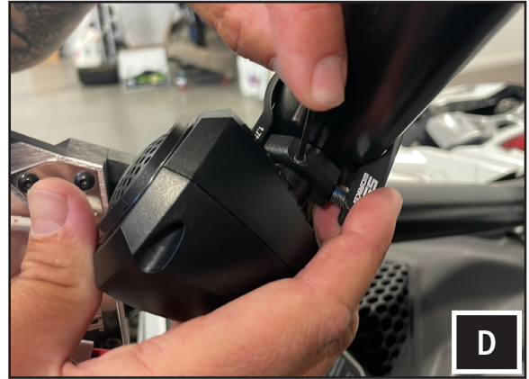
D. Insert the tweeter pod post into the swivel mount and loosely tighten the set screw using the provided 2mm Allen wrench.
