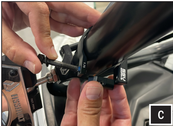
C. Install the swivel mount to the clamp using the M6 allen socket head bolt and washer with a 5mm allen key. Do not fully tighten yet.
