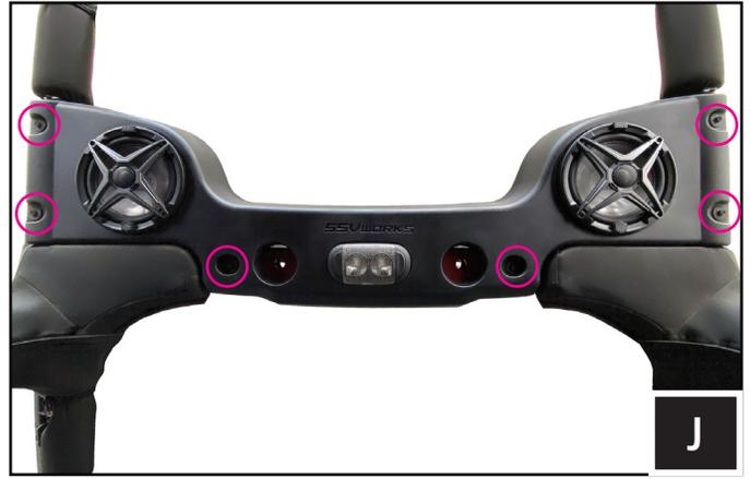
J. Using the factory x6 Bolts secure the new soundbar to the vehicle roll cage.
