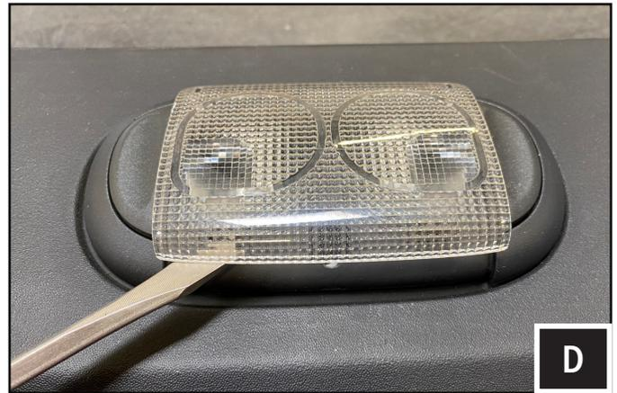
E. Using a panel removal tool or flat head screwdriver, unsnap the plastic dome light lens.
