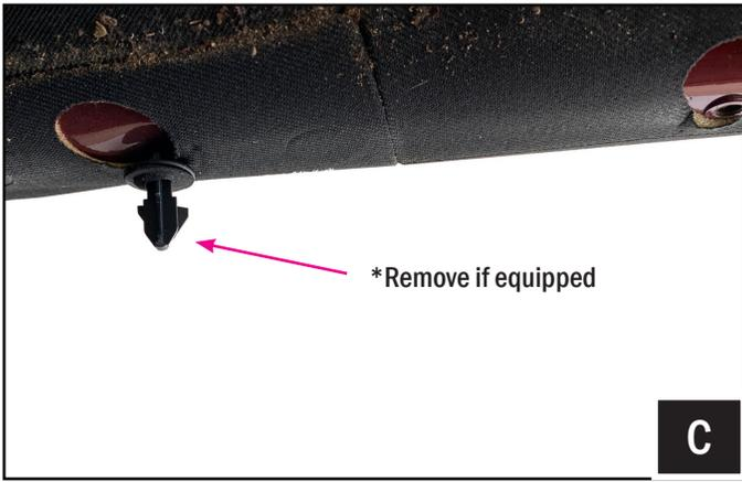
C. Once the factory soundbar has been removed use a panel removal tool and extract the plastic locating pin. These will not be needed for the new soundbar.
