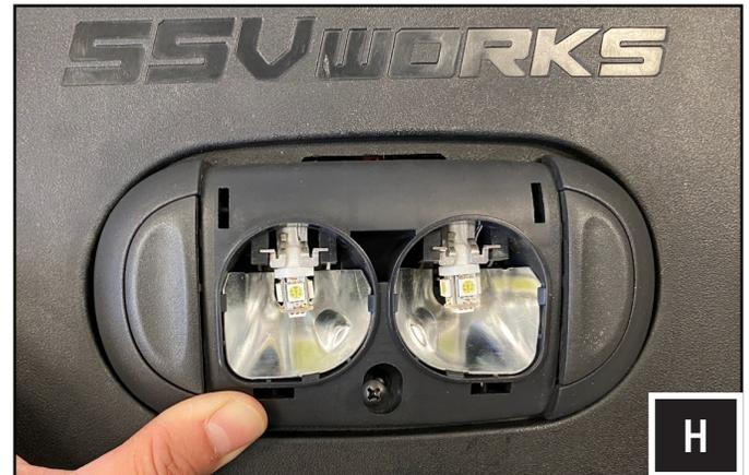
H. Hold down the domelight while fastening the provided SSV Works #2 Phillips screw to secure the dome light down to soundbar.
