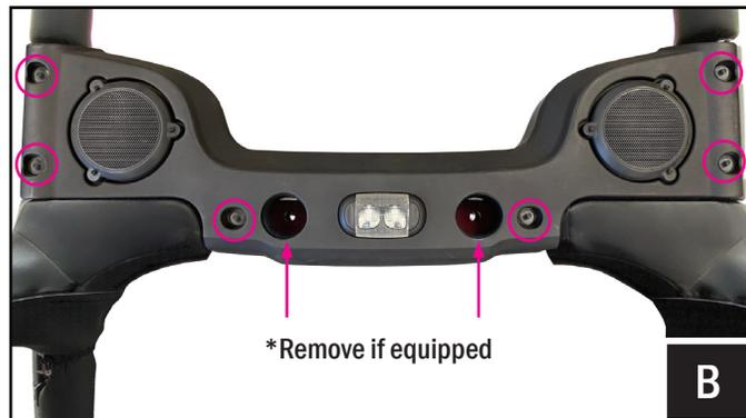
B. Extract the x6 Bolts securing the enclosure to the vehicle roll cage and set aside for use on the last step. If your vehicle is equipped with a top remove the two hand threaded cups along each side of the dome light. Remove the soundbar from the vehicle.
