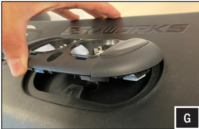
G. The SSV soundbar is made thicker than the factory soundbar to support the 8" speakers. The dome light will fit tight because of this. Angle in the dome light so both plastic tabs hook onto the material first then push in and lay flat.
