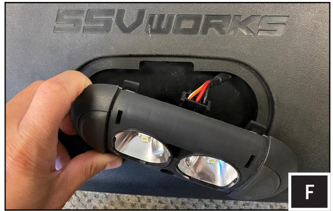
F. Connect the factory dome light into the SSV soundbar.
