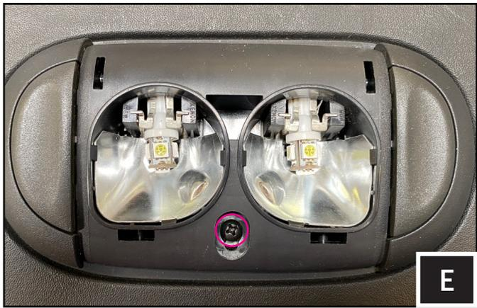
E. Extract the screw securing the dome light to the sound bar.
