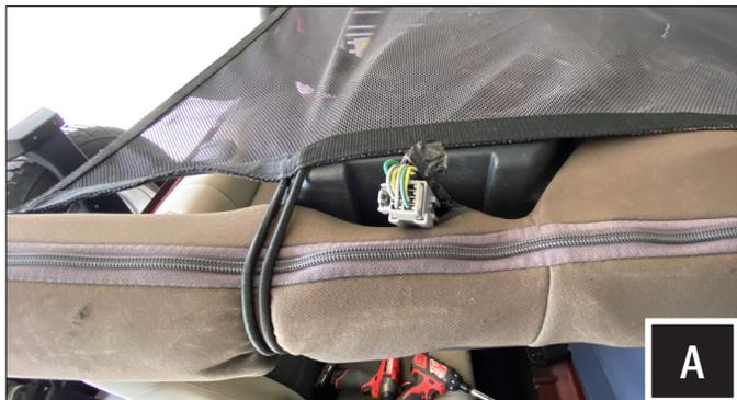
A. From the passenger side of the vehicle locate the connector at the top of the soundbar and disconnect.
