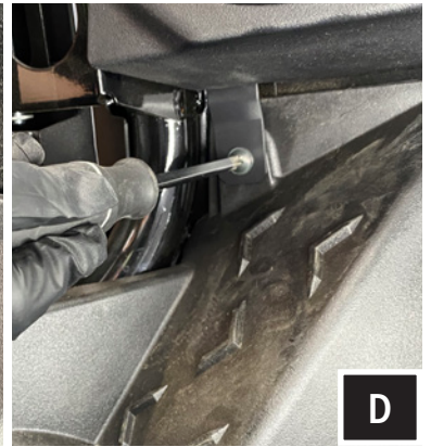
D. Starting on the drivers side, Remove the factory screw at the top of the footrest. Place the speaker pod in position and use the same factory screw to attach the bottom bracket.
