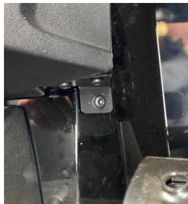
H. Connect Bracket "C" by pushing the 25mm M6 screw through the drilled hole and hand tighten the locking nut from the other side of the floorboard. It is recommended to have 2 people complete this step, one person on each end of the screw as it is tightened.
