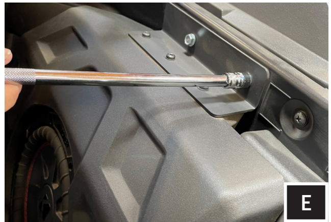
E. Tighten bolts on back wall.
