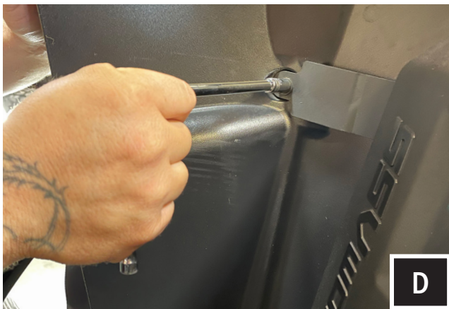
D. Place sub enclosure back in its designed location, place plastic spacer between sidewall of machine and side bracket. Tighten bolt down.
