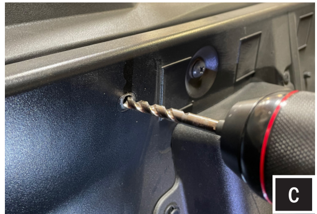
C. Pull enclosure away and finish drilling.
