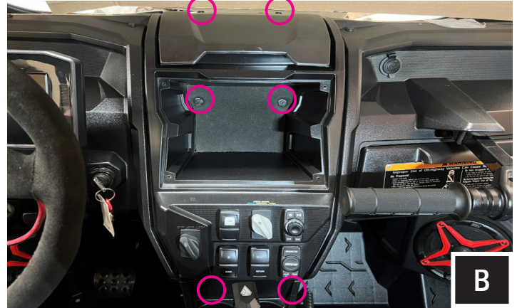
B. Remove 4 panel clips and 2 Phillips screws.
