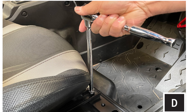
D. Remove the seat, use a 13mm socket and wrench to remove front (2) bolts and nuts. Use an 18mm socket to remove (2) rear nuts and seat belt nut (repeat on other seat).
