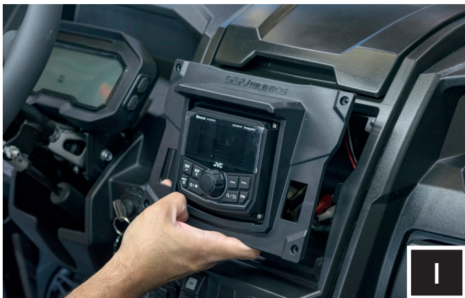
I. If desired, you can add another rocker switch accessory switch at this time. Insert the head unit and B-D2449 dash kit into the dash panel
