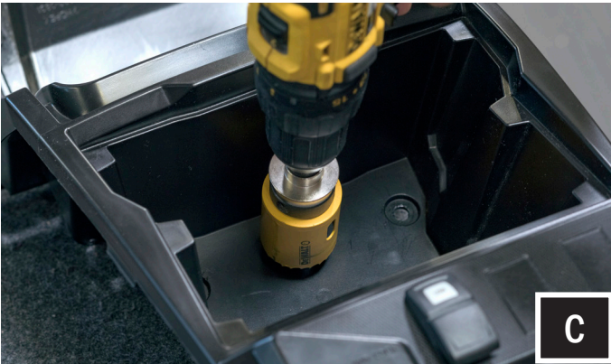
C. Drill 1 5/8" to 1 3/4" hole in the back of the pocket of the dash panel
