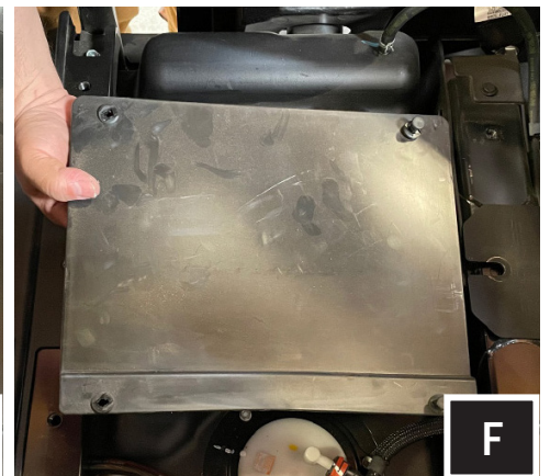
F. Using clip removal tool, unclip the (4) clips and remove fuel pump cover.
