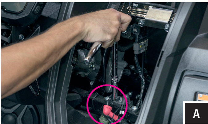
A. Attach the positive and negative ring terminals from B-H2367 harness to the accessory and ground posts mounted on the cross bar behind the dash
