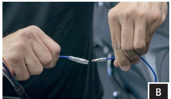
B. Connect the remote wire from the B-H2367 harness to the remote wire of the B-H2605 Amp harness using the pre terminated bullet connectors
