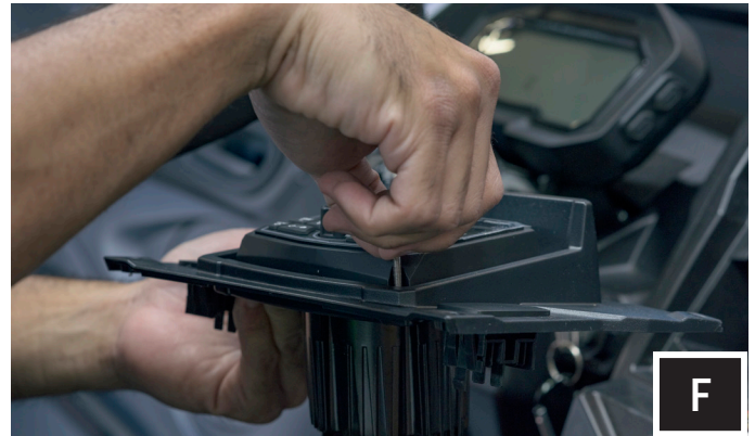
F. Secure the headunit to the dash kit and backing plate with the 4 phillips screws provided with the headunit
