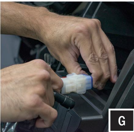
G. Connect the head unit into the B-H2367 harness previously installed in the dash pocket
