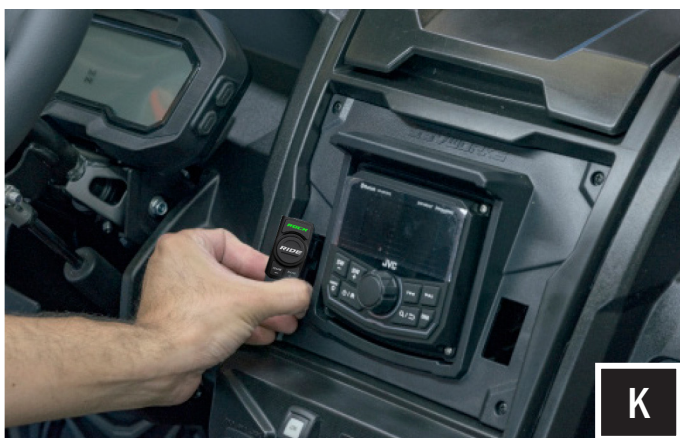
K. Insert the Rock and Ride Rocker switch and a BO-Y-RSB switch blank into the dash kit openings.
