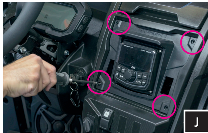
J. Secure the B-D2449 dash kit to the dash panel using 4 philips screws
