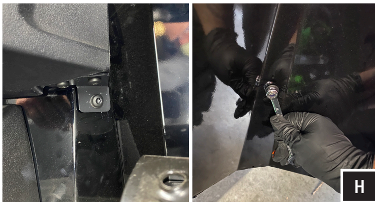
H. Connect Bracket "C" by pushing the 25mm M6 screw through the drilled hole and hand tighten the locking nut from the other side of the floorboard. It is recommended to have 2 people complete this step, one person on each end of the screw as it is tightened.
