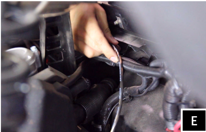
E. Route the Audio (B-1913 & B-H1912) and RGB extension harnesses (B-H2933 & B-H2934) along the factory wires in the engine compartment and pull up through the small space between the bed panel and cage tubing on both passenger and driver sides.
