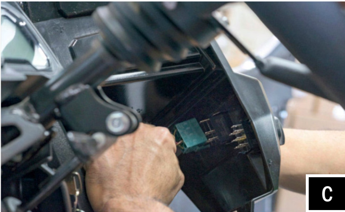
C. Remove the dash panel and unplug the drive selector and gear selector switches
