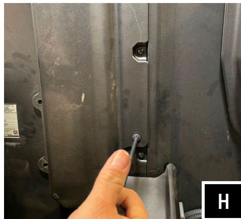
H. Remove phillips screws and panel clips to remove the center panel on the back wall.
