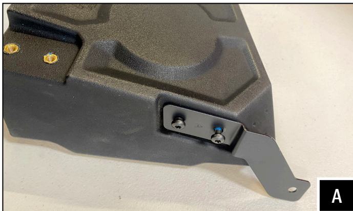
A. Attach Bracket "A" to the driver side pod and Bracket "E" to the passenger side pod as shown using two (2) M6 screws and washers.
