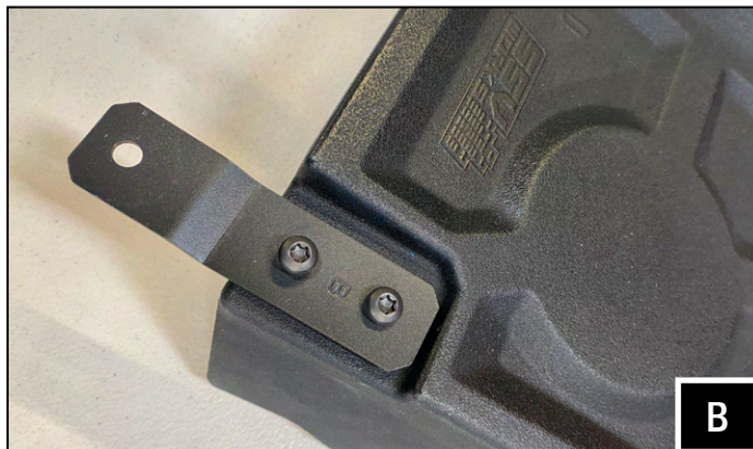
B. Attach Bracket "B" to the driver side pod and Bracket "F" to the passenger side pod as shown using two (2) M6 screws and washers.
