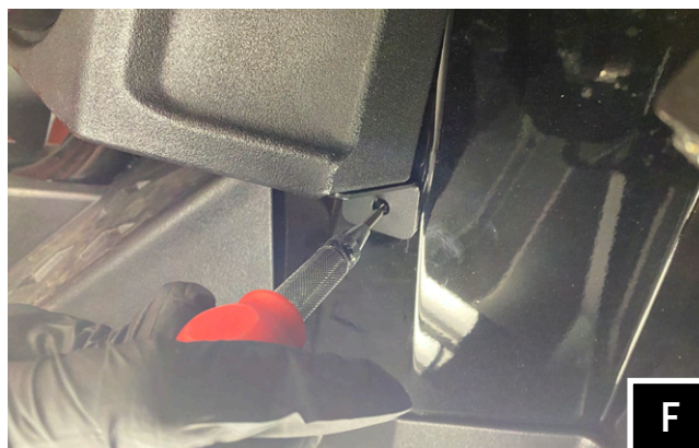
F. Using a punch tool, create a drill guide at the center of Bracket "C" hole.
