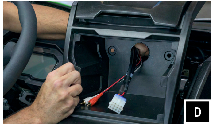
D. Reconnect the drive selector and gear selector switches from Step B. Run the Power Harness (B-H2367) white multi-pin connector through the previously drilled hole. Reinstall the dash panel including push pins and screws.
