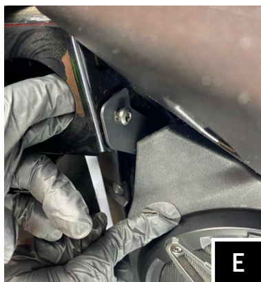
E. Place Bracket "D" through the door jam hole (as shown above) and use a M6 screw and washer to attach Bracket "A"
