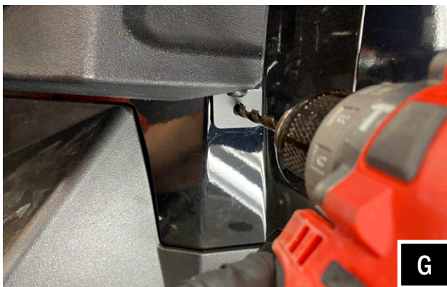
G. Using the guide left by the punch tool, drill a hole using a 1/4" drill bit
