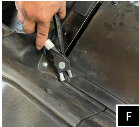
F. Using clip removal tool, unclip the (4) clips and remove fuel pump cover.
