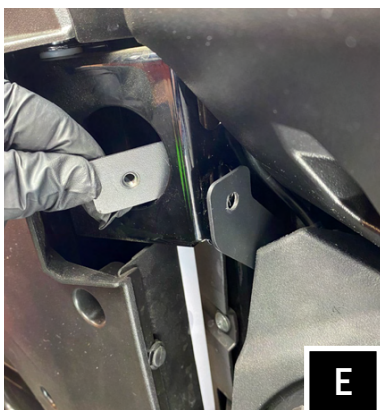
E. Place Bracket "D" through the door jam hole (as shown above) and use a M6 screw and washer to attach Bracket "A"
