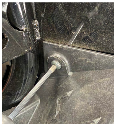
D. Starting on the drivers side, Remove the factory screw at the top of the footrest. Place the speaker pod in position and use the same factory screw to attach the bottom bracket.
