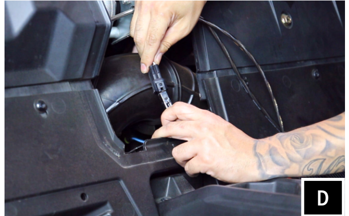
D. Take the B-H2936 RGB rear speaker harness and plug into the B-H1913 & B-H1912 audio extension harnesses and to the B-H2933 & B-H2934 RGB extension harnesses.
