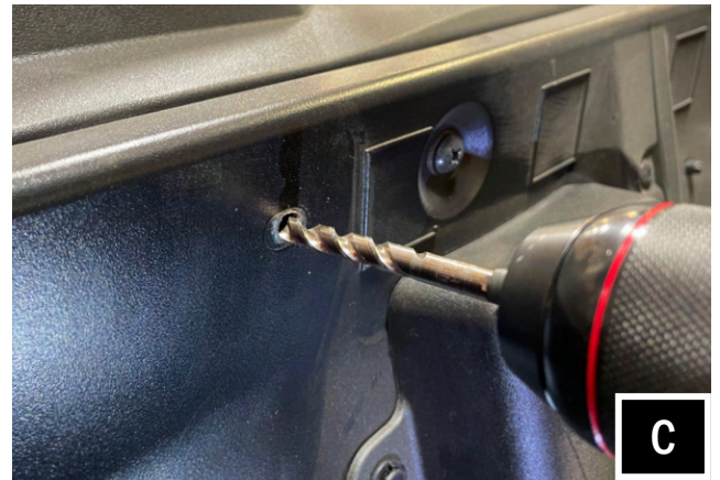
C. Pull enclosure away and finish drilling.
