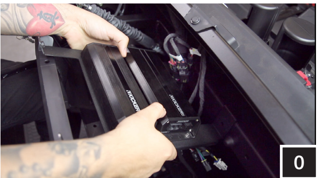
O. Move the factory wiring to the rear of the dash cavity. Place the mounting plate in the former location of the factory bracket.
