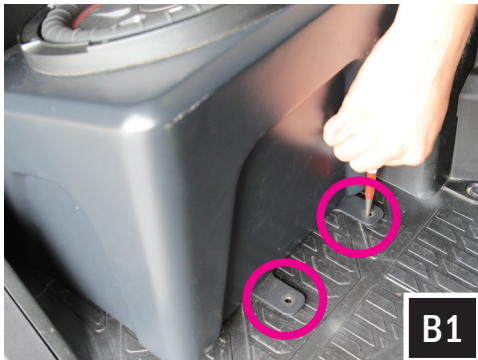
B1. With the brackets seated into one another, use the front mounting tabs as a template to mark with a scribe or punch the needed placement to drill pilot holes.
