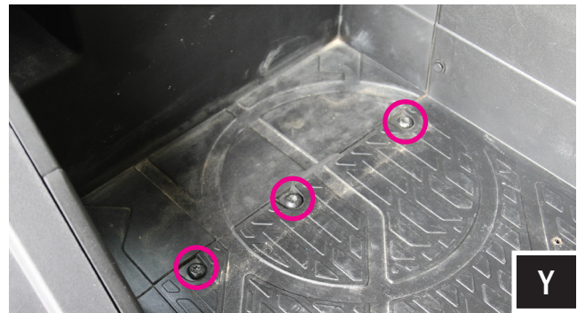
Y. Located on the floorboard to the right of the battery compartment, remove the (3) T40 torx screws circled in pink.
