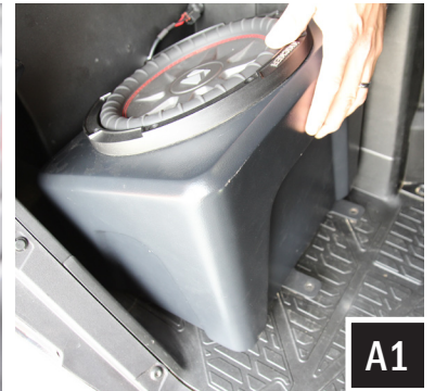
A1. With the bracket secured to the floorboard, place the enclosure in front of the floorboard bracket. To allow proper engagement, tilt the enclosure back slightly and slide its bottom bracket into the floorboard bracket catch.
