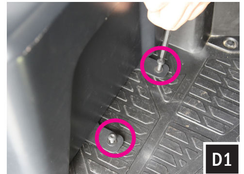
D1. Re-install the sub-enclosure. Secure the front mounting tabs with the kit provide T30 torx self-tapping screws.
