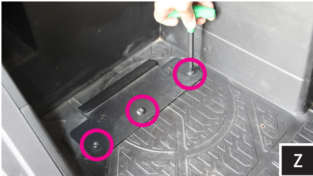
Z. Place SSV bracket B over the factory screw holes and refasten down with the (3) factory T40 torx screws removed in the previous step.
