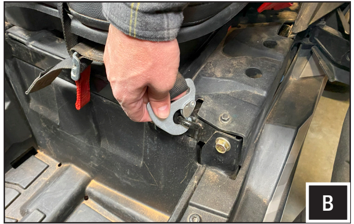
B. Detach seat belts to gain access to the bottom seat tray.
