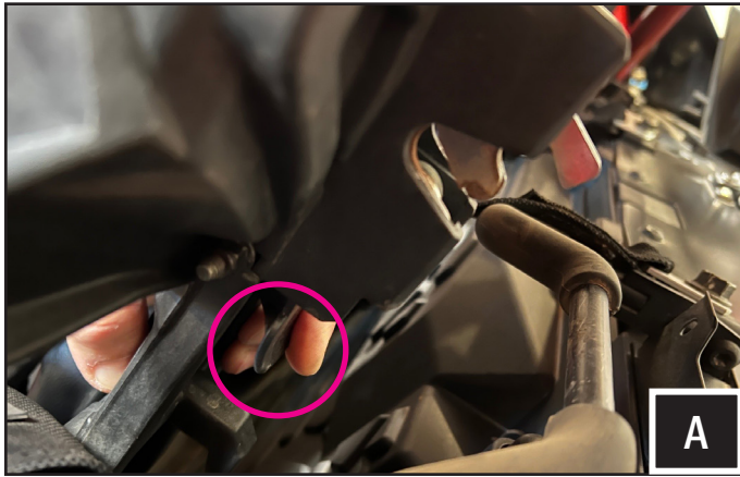
A. Depress the lever behind the headrest to release the backrest.
