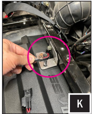
K. Once all bracket screws are installed, tighten the screws using a 15mm and 8mm socket and/or box wrench.
