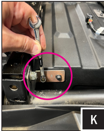
K. Once all bracket screws are installed, tighten the screws using a 15mm and 8mm socket and/or box wrench.
