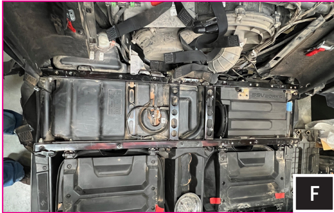
F. Remove the H bracket using a 15mm socket and box wrench.
