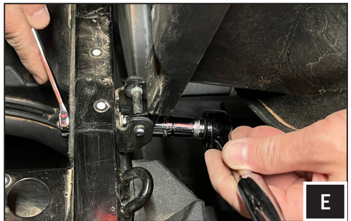
E. Remove the (2) seat bolts using a 13mm socket and box wrench. Remove the seat bottom. Repeat the process on the other seat bottom.
