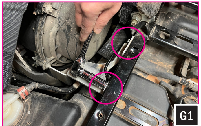
G. There is a heat shield bolted to the H bracket. Some models use (2) T40 Torx screws [G] and some use (2) 10mm hex head screws [G1] to secure the heat shield. Remove these screws to release the H bracket.
