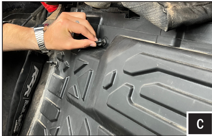
C. Twist the spring clips on the firewall to remove the top and bottom firewall panels.
