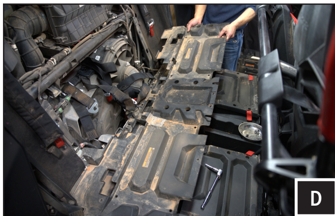
D. Remove the screws holding the bottom seat tray using a T40 Torx driver.
