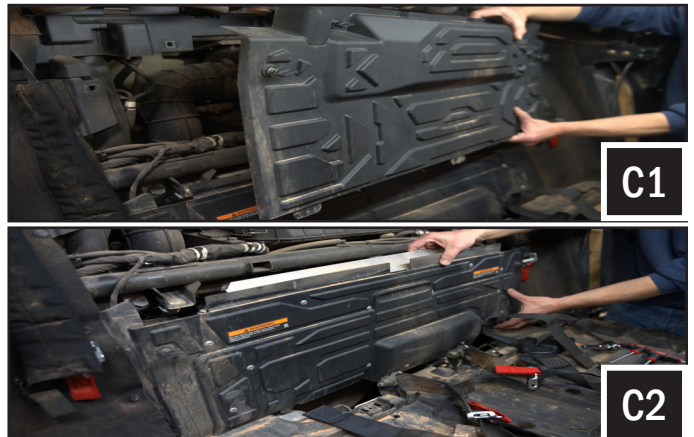
B. Detach seat belts to gain access to the bottom seat tray.
