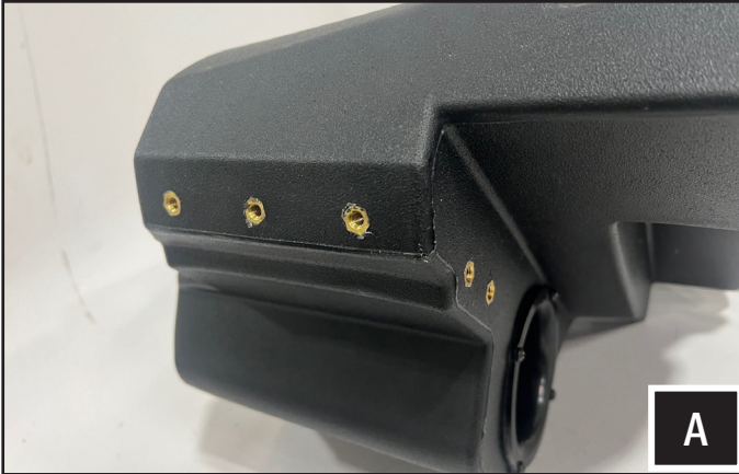
A. Secure the base bracket to the enclosure with (5) M6x1.0x12mm T30 screws and washers.
