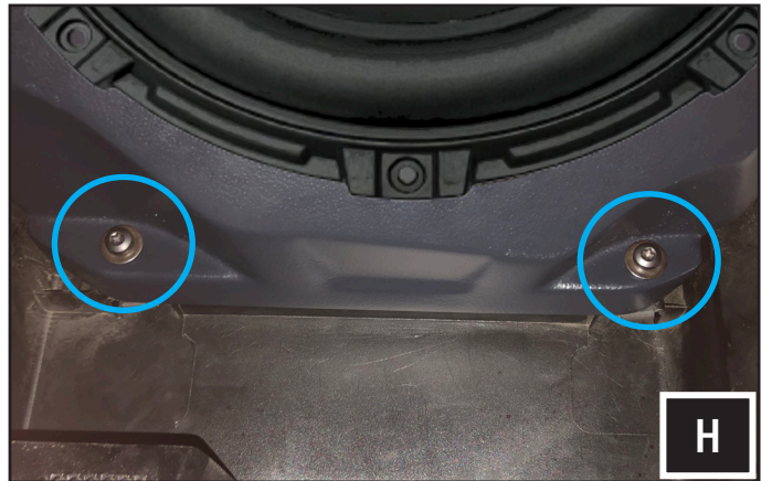
H. Secure the bottom of the enclosure with the provided M6x1.0x40mm T30 screws and washers to the M6 clip nuts attached to the firewall.
