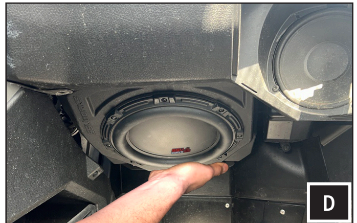
D. Apply force to the bottom of the enclosure to swing it up into place. Once it is in place the lower mounting points will be in-line with the (2) M6 clip nuts.
