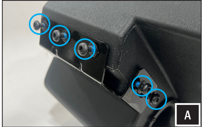
A. Secure the base bracket to the enclosure with (5) M6x1.0x12mm T30 screws and washers.
