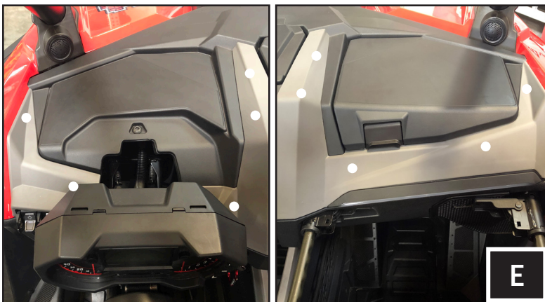
E. Use a panel tool to assist with the removal of the (3) trim panels. The white highlighted points represent the location of the panel clips that are retaining the trim panels to the dash.
