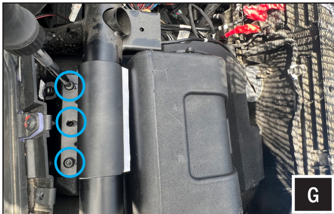
G. Secure the clamp bracket to the base bracket with (3) M6x1.0x12mm T30 screws and washers.
