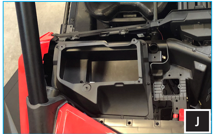
J. Lift and remove the glove compartment from the dash cavity.
