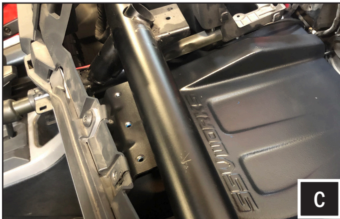
C. The top of the enclosure will tuck under the chassis cross bar. The bottom of the enclosure will rest above the edge of the firewall.
