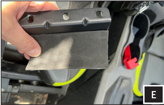
E. Stick the included foam piece to the clamp bracket.
