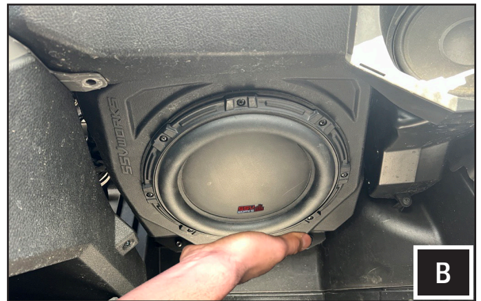
B. From the passenger footwell, lift the RZ5-UD10 into the dash cavity.
