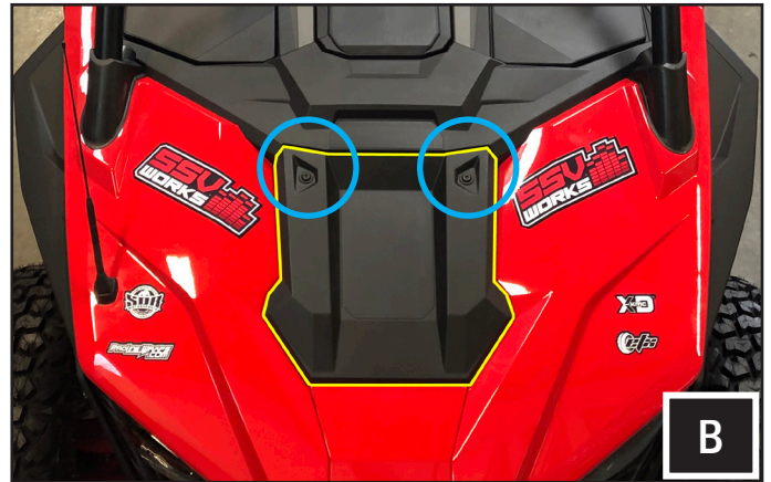
B. Remove the (2) T40 torx screws that holds the center hood panel.
