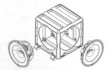
Position of SUBWOOFER and PASSIVE RADIATOR are interchangeable
