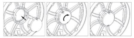
The above diagram shows the installation of the tweeter. Insert & rotate the tweeter clockwise. The removal of the tweeter is the opposite.
