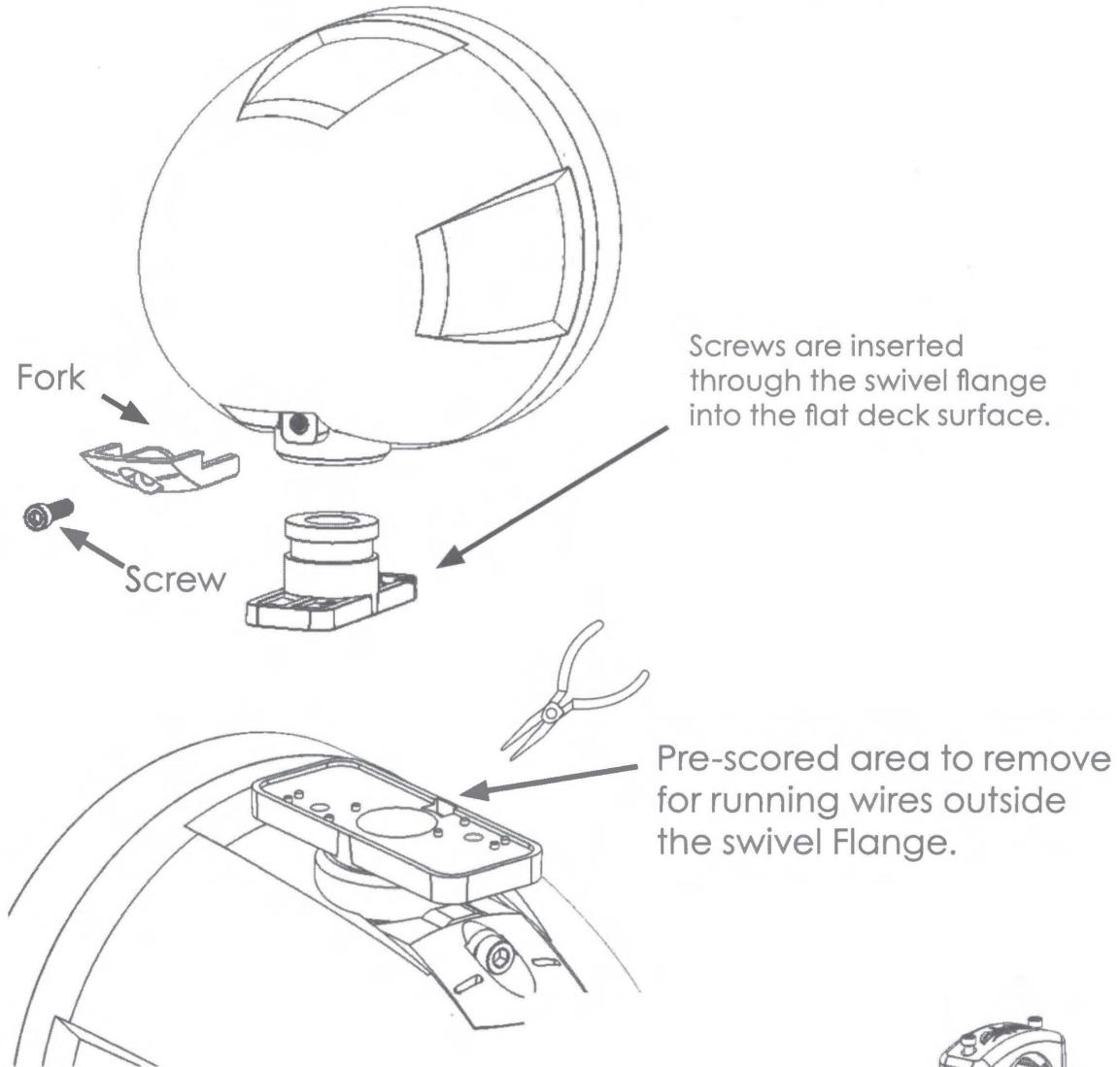
If mounting the Pod at an angle or inverted, simply remove the 4 Philips head screws holding the speaker in the Pod, then rotate the speaker so that the grill is straight. Then re-insert the 4 screws.
