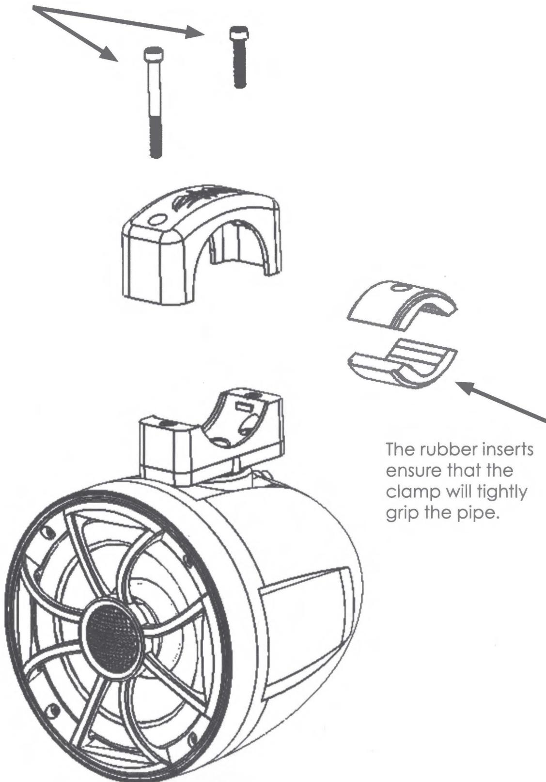
Speaker/RGB wires may be inserted from the top of the Pod through the center of the Swivel Flange & Bottom clamp, then through a hole in the mounting surface or pipe. To run the wires without drilling a hole in the surface or pipe, there is a pre-scored area on the side of the Swivel Flange & the bottom clamp to remove, allowing the wires to pass through.
