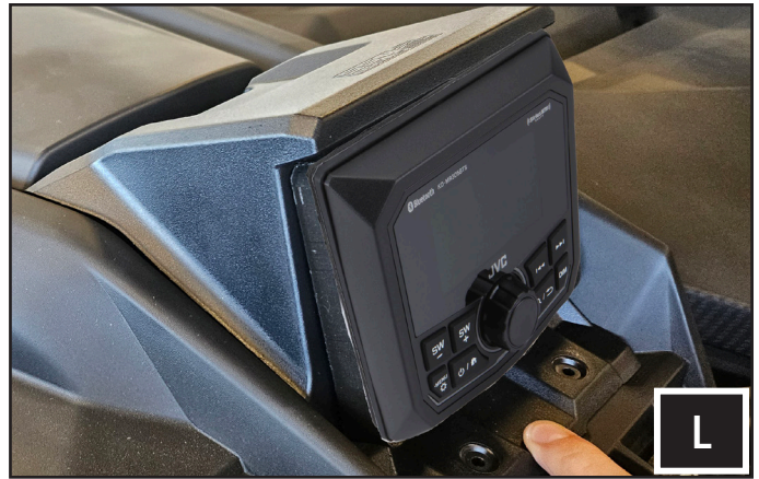
L. Plug the radio connect connectors to the mating harness and set the dash panel on the dashboard.
