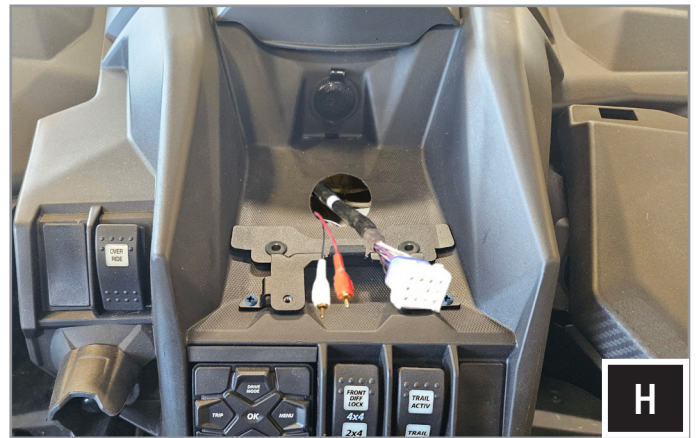
H. Make the radio harness connections and run the connectors through the dashboard hole.
