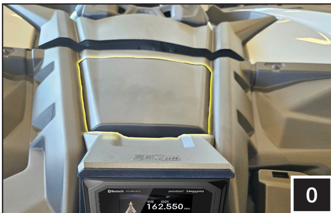
O. Reinstall the top compartment cover.
